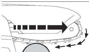
If the moving cutting chain hits a hard object and stops quickly, the wood cutting machine may suddenly be pulled out by the user. People can be injured.
