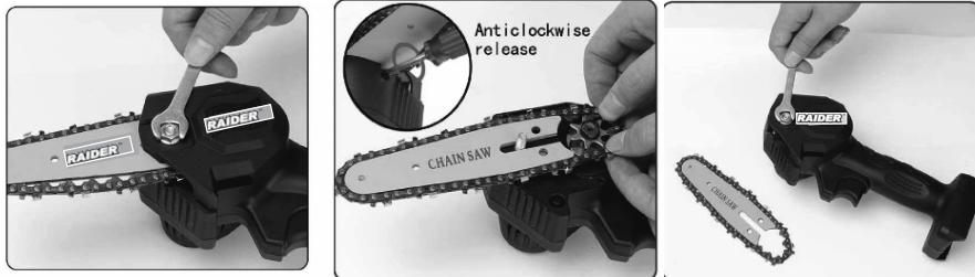
Before mounting the guide bar and the cutting chain, you must check the correct position of the cutting blades on the chain (the correct position of the chain on the bar is shown on the front of the bar). Wear protective gloves when inspecting and installing the chain to avoid injuries from sharp cutting edges.
