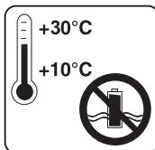
Store the battery only in dry rooms with an ambient temperature of +10°C to +30°C.
